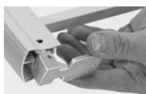
**Step 12.** Use a 13/64" diameter drill to align holes in end bracket to holes in top rail.
