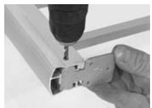
**Step 13.** Insert a 1-1/4" long, slotted truss head #8 female binder bolt. Turn male binder bolt screw into female binder bolt and tighten to secure assembly together. Follow the same procedure on opposite end of top rail.
