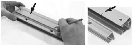
**Step 1.** Position bottom rail against top rail and align ends so they are flush with each other. With a pencil draw a line on top rail, just above each hole of the bottom rail.
