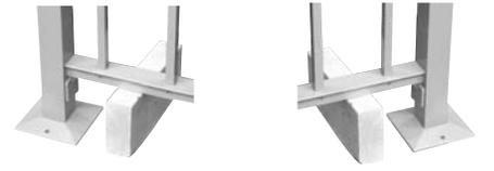
**Step 2.** When required railing height is achieved, position post against railing end brackets. Using holes in end brackets as a template, mark each mounting hole location. Mark the hole locations at top, bottom and on each rail section end. See "Note" below.
