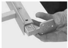
**Step 15.** Use a 13/64" diameter drill to align holes in end bracket to holes in bottom rail, as shown in Step 12. Insert a 15/16" long, Phillips truss head #8 female binder bolt, through the bottom rail and end bracket. Secure the assembly together by inserting and tightening a male screw into end of binder bolt.
