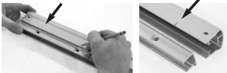
**Step 1.** Position bottom rail against top rail and align ends so they are flush with each other. With a pencil draw a line on top rail, just above each hole of the bottom rail.
