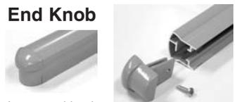
Insert end knob into top hand rail, then insert screw into end knob. Tighten screw to secure end knob in place.
