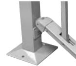
**Note:** Before pencil marking swivel bracket holes on post, check that post base mounting holes are facing in opposite directions to railing sections as shown in photo at left. The reason for this is that it is easier to install post base mounting bolts. Disregard this "Note" for railing corner post.
